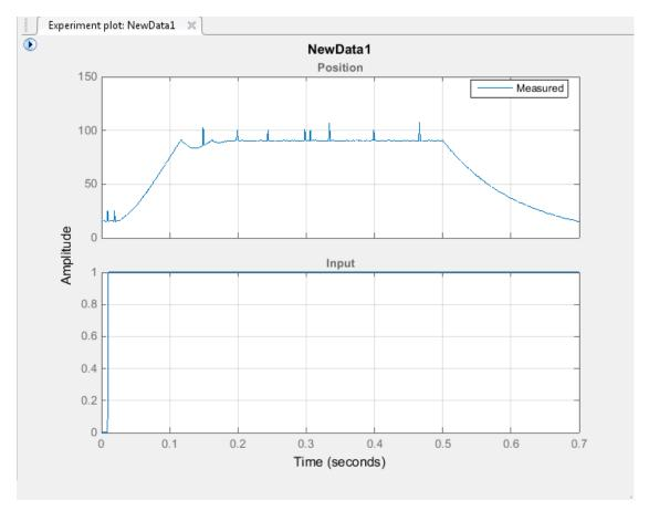
The time plot shows the output data in response to a step input, as described in "About the Sample Data" on page 2-4. The plot shows a rapid decrease in the response after t=0.5 s because the system is shut down. To focus parameter estimation on the time period when the system is active, select the data samples between t=0 s and t=0.5 s, as in "Extract Data for Estimation" on page 2-9 .
