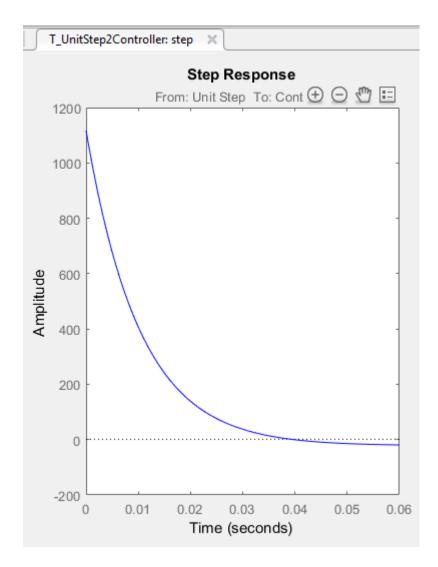
The plot shows that the peak value of the controller output is about 1100, which is large and can damage the plant. To limit the controller output, apply lower and upper bounds on the signal, as specified in "Design Requirements" on page 4-16.
